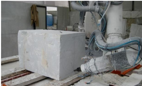
Robot milling makes quick work of reducing a marble block into highly detailed and complex shapes, based on 3D digital matrix information.
